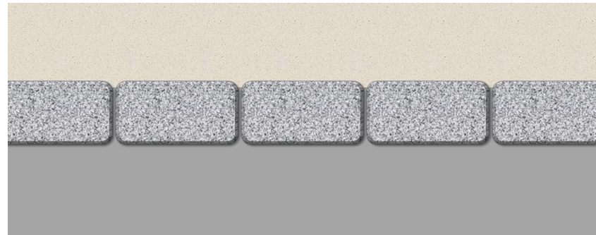
Figure 1. String course of granite setts, set into carriageway
